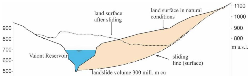
Fig. 4. Catastrophic landslide in Vaiont Reservoir - cross-section (Selli et al. 1984).
